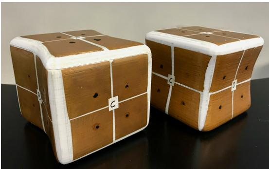
Figure 2: Objects covered with copper pads connected to an electronic board placed inside. Each face is tagged with a letter.
